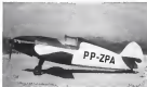
ECHINO , another Beechcraft design, is powered by a Continental 75 hp engine. Like the T-PF 31, it is a wood construction with plywood covering. Span is 22 ft., stalling speed, 120 mph.
